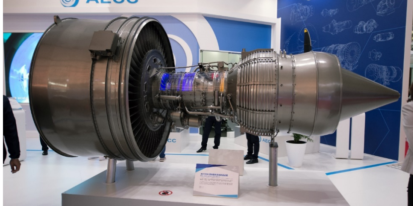
AECC AEF3500 Wide-Body Passenger Aircraft Engine on Display at MAKS 2019 119
