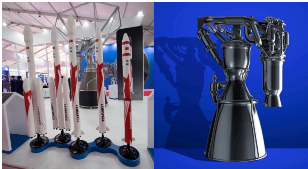
Zhuque (ZQ) Family of Rockets (left) on Display and Tianque 80-ton Liquid Oxygen Methane Rocket Engine (right) on Display and from Brochure at MAKS 2019 199
