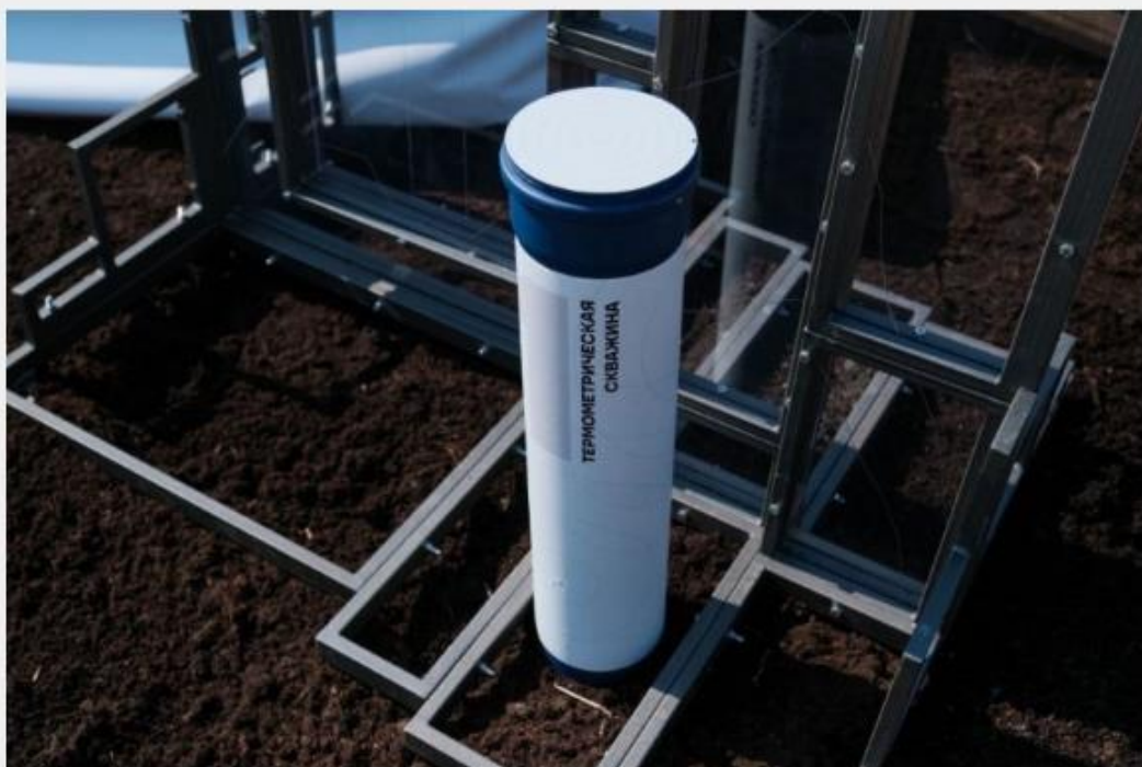
The first bore hole of the permafrost monitoring system in the Russian Arctic. Photo: Ministry of Natural Resources of the Russian Federation
