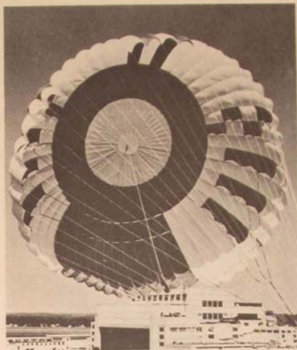
A 51-foot-diameter parasail parachute, developed for high-altitude cargo drops, is static-tested by Air Force Flight Dynamics Laboratory engineers. The parasail can be guided automatically or manually into an impact zone and homes on signal from a ground transmitter.
