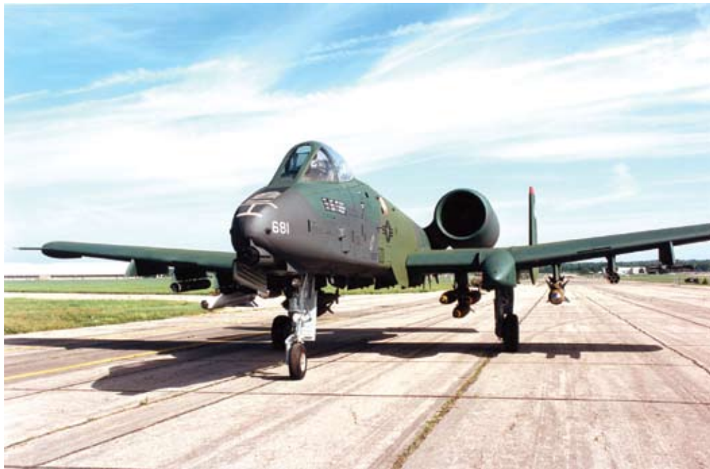
Figure 77. Fairchild-Republic A-10 "Hog," stalwart of close air support in Desert Storm and after, armed with 30 mm Gatling gun. (USAF photo)
