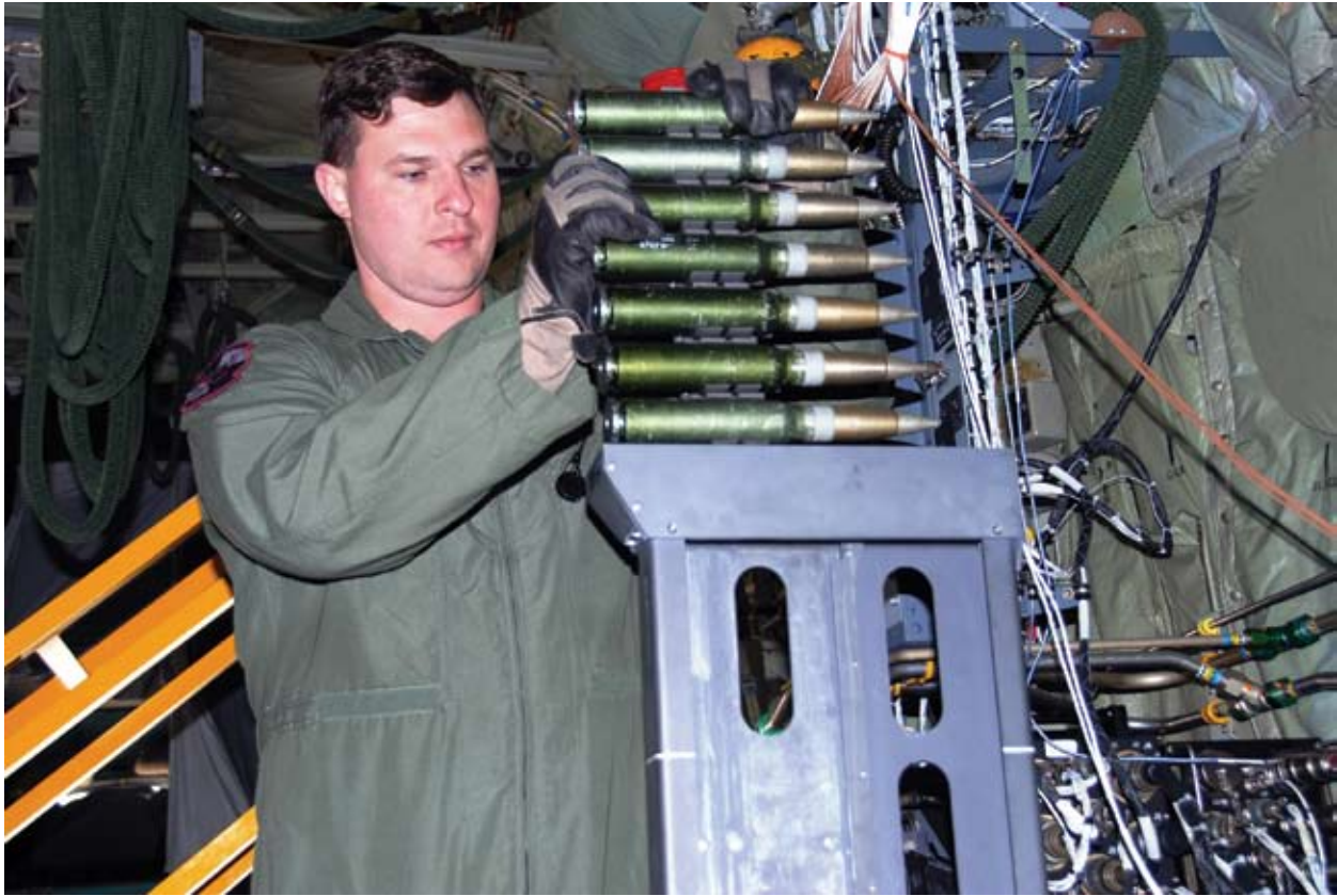
Figure 75. TSgt Ben Filek loading the 30mm gun on an AC-130. (USAF photo)
