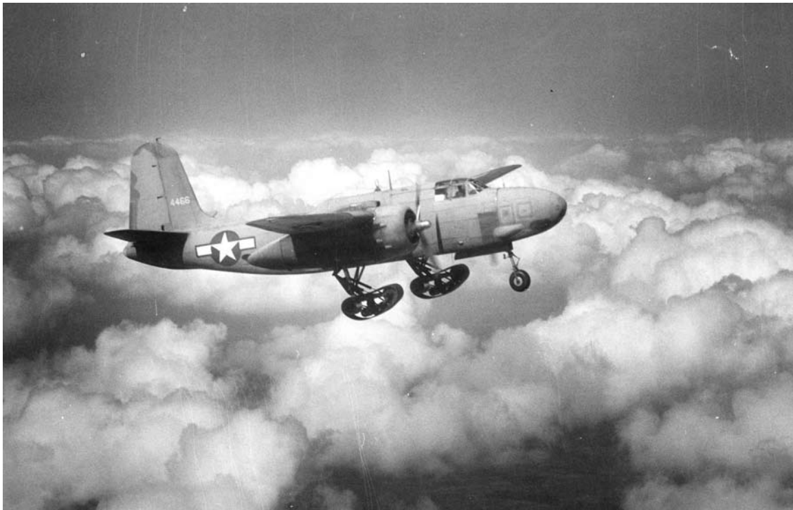
Figure 36. The A-20 Invaders in New Guinea operated under very primitive conditions. Later in the war, experiments were run with tracked landing gear, as shown here, to enable operations from unprepared runways. (USAF photo)
