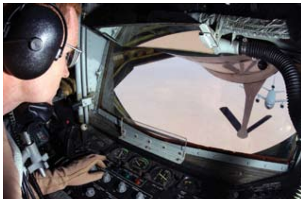
Figure 56. Boom operator MSgt Sam Blackwell prepares to transfer fuel to a KC-10 Extender. (USAF photo)
