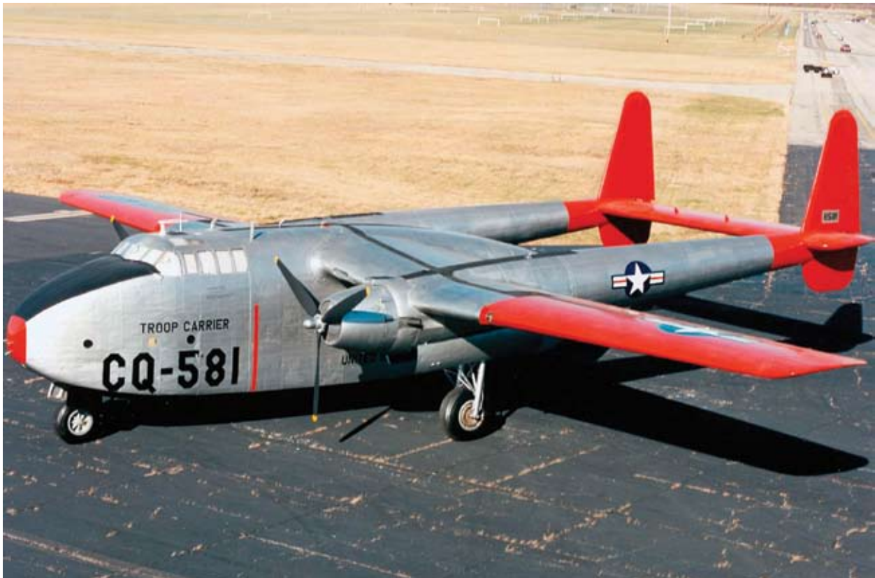
Figure 44. Fairchild C-82 Packet. Only a few participated in the Berlin airlift, but they were vital because they could be loaded with equipment that could not be handled by other aircraft. (USAF photo)
