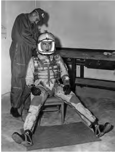
Figure 2.3. James A. Howell suits up for the “human subject” test of the F-106B ejection seat, 6 June 1961. Howell “jumped” from an altitude of over 22,000 feet and indicated airspeed of 560 knots. (Photo courtesy of James A. Howell.)
