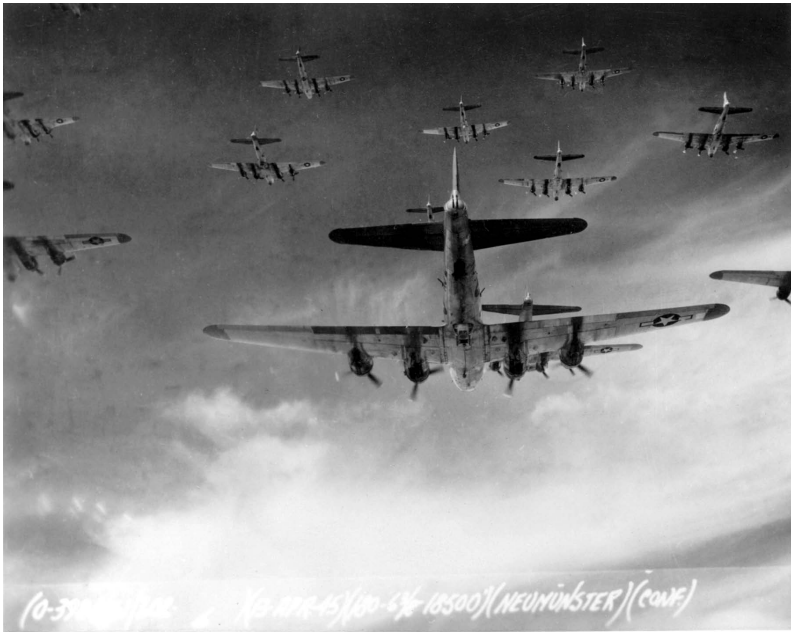
Fig. 9. During the Combined Bomber Offensive, B-17s flew in a “combat box” formation to increase defensive firepower. All total, 11 aircraft flew in very close proximity with the idea that each bomber’s 10, .50-caliber machine guns could cover itself and other bombers. This photo (taken from an aircraft in the rear of the formation) is from a 13 April 1945 mission to bomb Neumünster, Germany. Courtesy of AFHF/NMAF.
