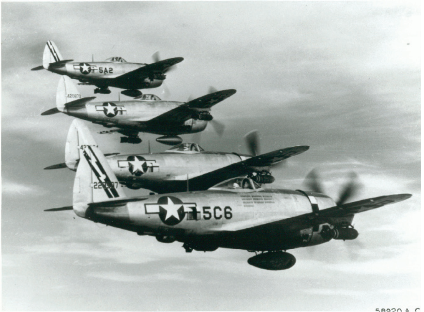
Late-model P-47s of the Twelfth Air Force have belly drop tanks and 500 pound bombs under their wings. This model has a much longer range than the P-47Bs used in 1943 and early 1944.
