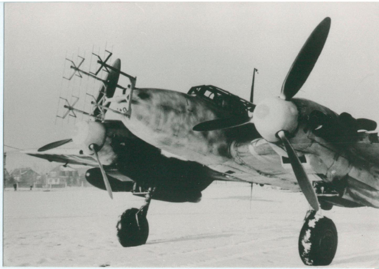
An Me-110 night fighter variant with nose radar array was a defender of the Reich.
