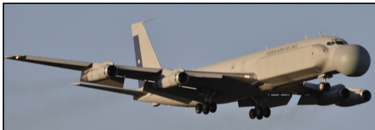
Phalcon System Integrated on a Boeing 707 for the Chilean Air Force
